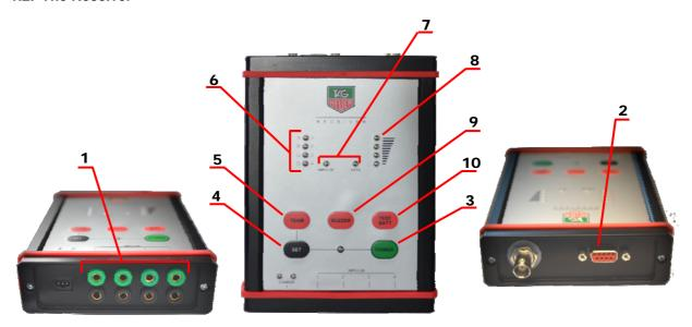
**1. IMPULSE** Output for timing Impulse (Start gate, photocell – working / closing contact). Respect the polarities.
