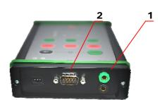
1. IMPULSE Input for timing Impulse (Start gate, photocell – working / closing contact). Respect
